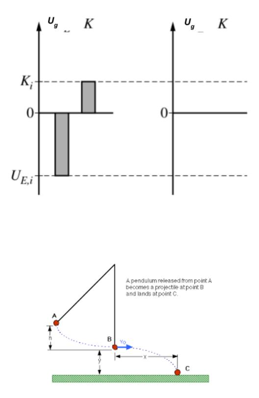
4. A 1.0 kg bob hanging from a 30 cm string is pulled back to point A and released. At point B, the string is cut and the bob becomes a projectile, eventually landing at point C. Drawing is NOT to scale!
