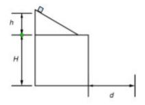
7. A student releases a block from rest from different vertical heights (h) on a smooth incline above the table top as shown above. The block slides down the ramp, then briefly slides horizontally across the smooth surface of the lab table of constant vertical height H cm before it is launched off the edge of the table. It then hits the ground a horizontal distance (d) away from the base of the table.
